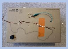
behind our steady hand game is that we will try not to make a circuit, so that a buzzer doesn't make a sound or a bulb doesn't light up. A platform for the box can be made out of cardboard.
